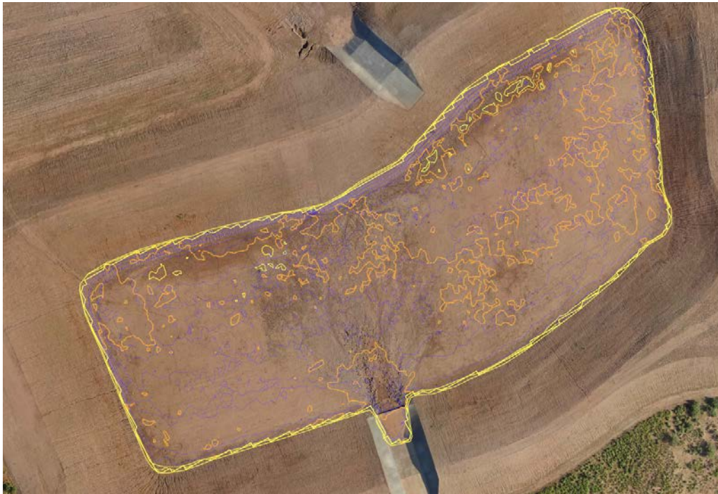
Figure 4. Basin Area Used for Volume (Cut/Fill) Report
